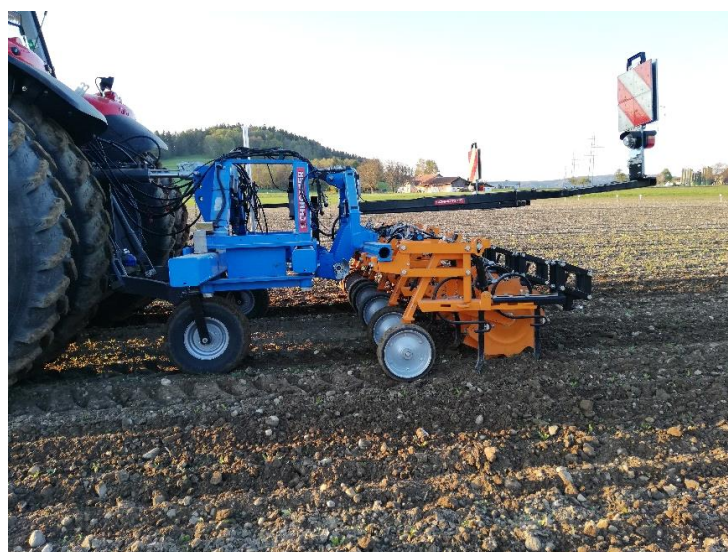
Figure 1. Camera-controlled hoe used for mechanical weed control on the trial plot of the SFF 2022 Weed Control Study in sugar beets.
