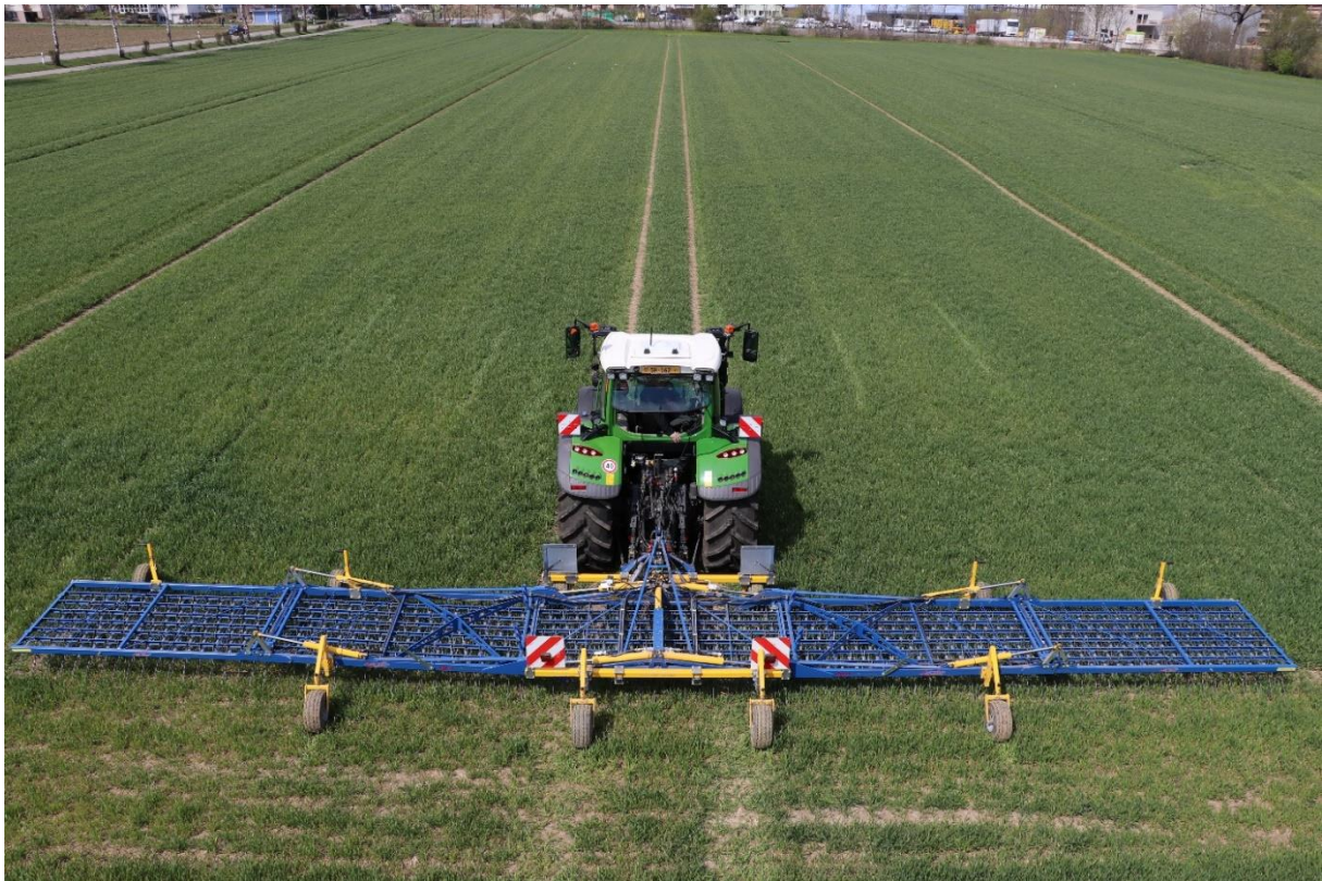
Figure 77. Tractor with tine harrow for mechanical weed control in winter wheat.
