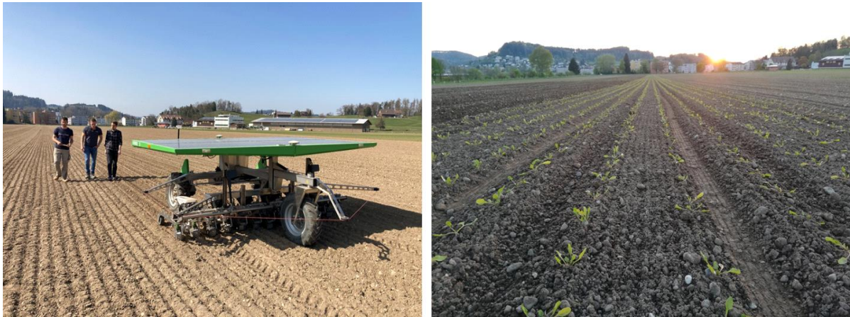
Figure 8. FarmDroid FD20 field robot planting sugar beets (left), transplanted beets on the day of planting (right) on the trial plot of the SFF 2022 Robotics & Transplanted Beets Study.
