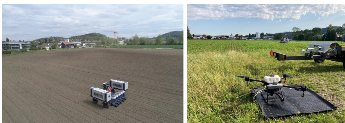
Figure 56. Agrobot 150D field robot with planter (left), DJI Agras T10 drone with sprayer unit (right) on the trial plot of the SFF 2022 Robotics & Autonomy Study in Silage Corn.
