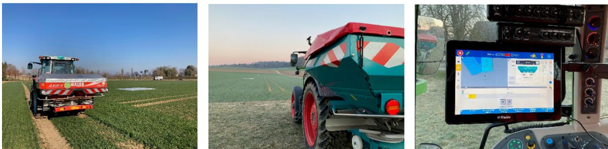
Figure 96: Tractors and fertilizer spreaders with automatic rate control via prescription map.
