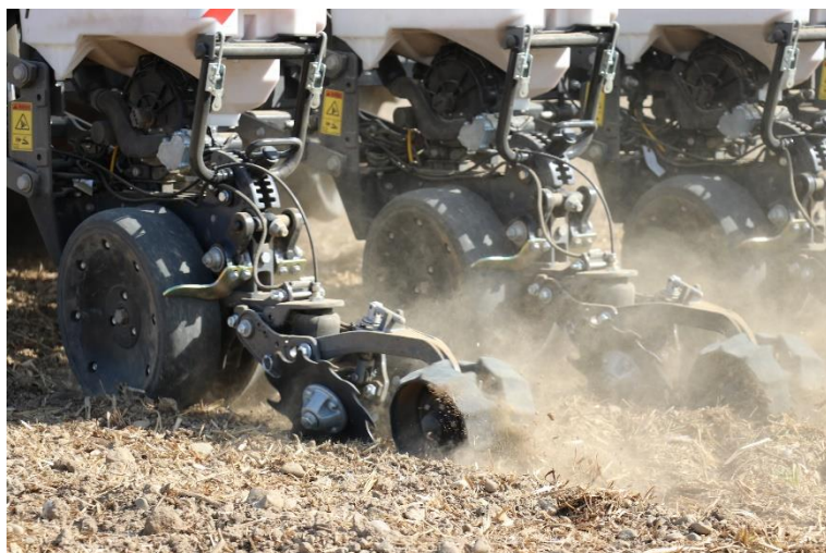
Figure 31. Precision Planting FurrowForce closing system on planter row unit.
