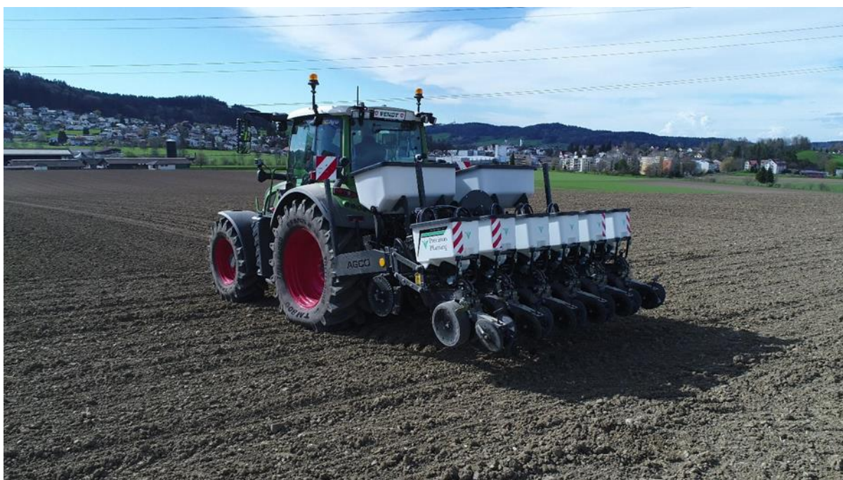
Figure 3. Precision Planting prototype planter during sugar beet planting at the Swiss Future Farm on 12 April 2018.
