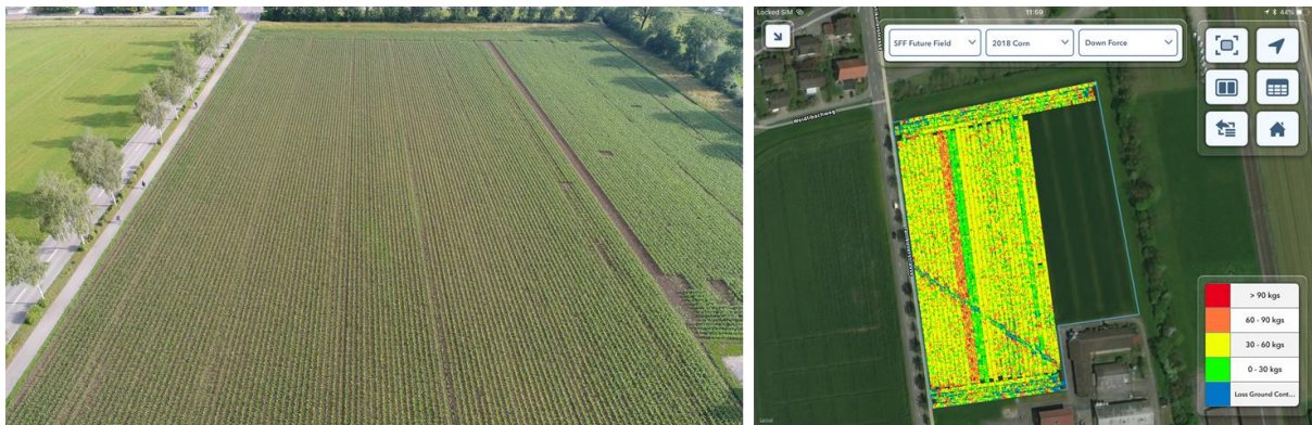
Figure 25. Down force measurement with Precision Planting DeltaForce and visualization in the Climate FieldView app with clearly recognizable compaction strip (blue) on the trial plot.
