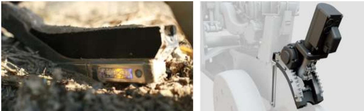
Figure 51. Precision Planting SmartFirmer for measurement of soil moisture in the furrow (left) and Precision Planting SmartDepth for real-time adaption of planting depth according to soil moisture content (right).
