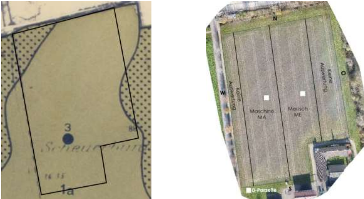
Figure 27. The soil zones are visible on the left side. The trial strips were laid out so that they all lie in the same soil zone as far as possible.
