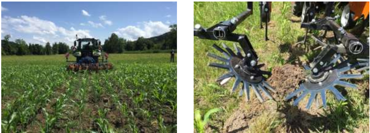
Figure 12. Pictures of the hoeing pass on June 21, 2021. The finger hoes in the right picture were dismantled because clods of soil were wedged in them.
