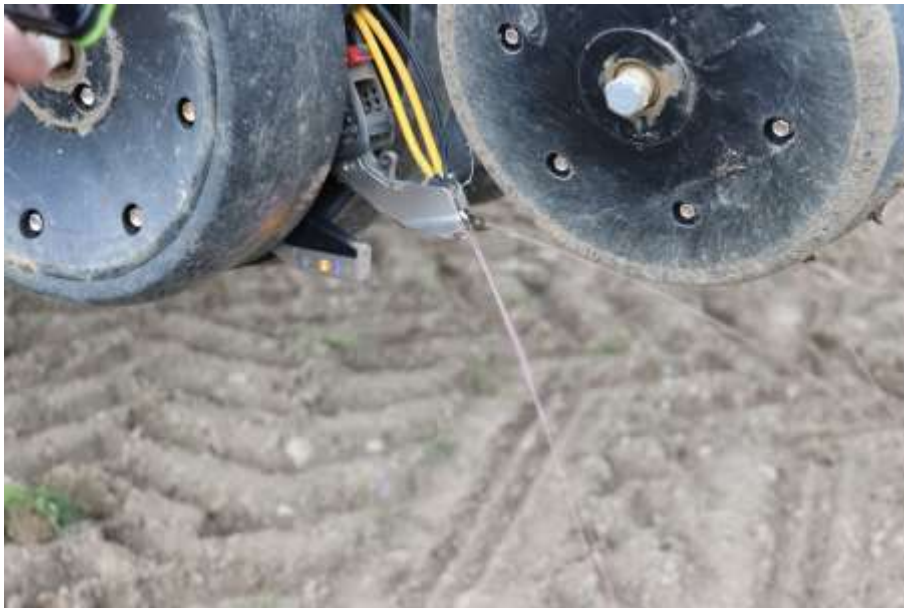
Figure 45. Precision Planting row unit equipped with FurrowJet liquid fertilizer system used for planting the trial plots.
