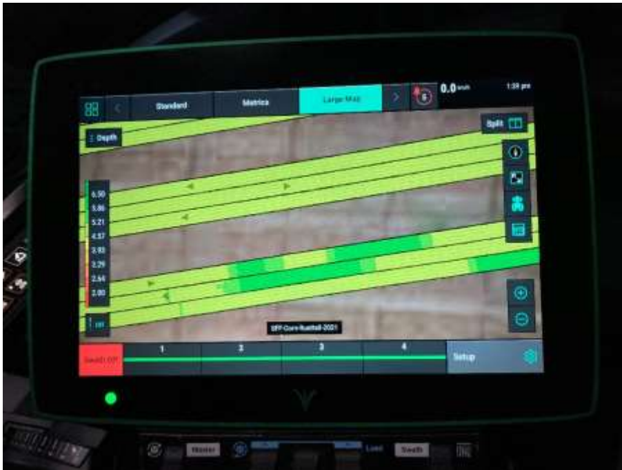
Figure 24. Uniform standard planting depth (planter passes on top) and variable planting depths (planter passes on bottom) on the trial field of the SFF 2021 Planting Depth Study in silage corn shown in the Precision Planting 20/20 Gen 3 monitor.
